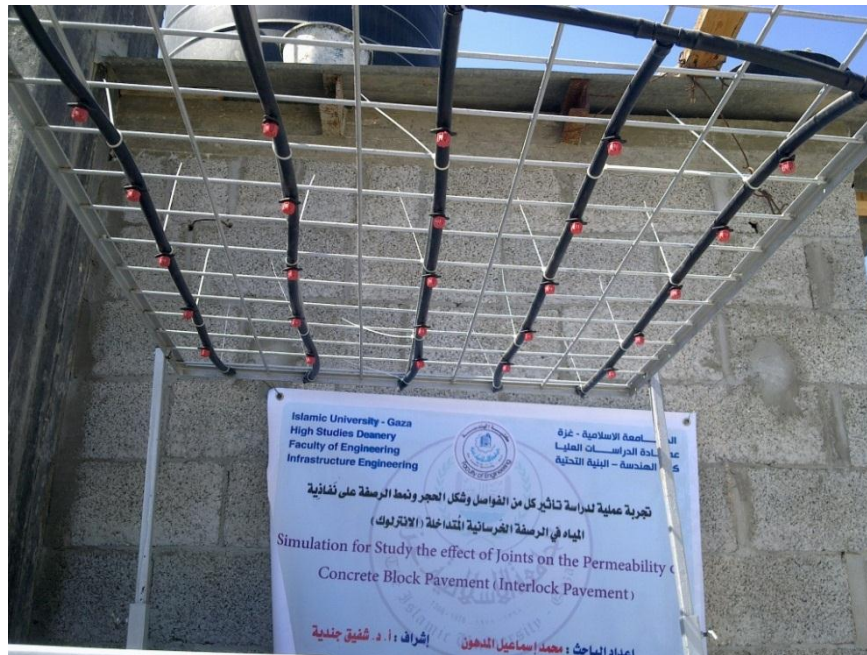
Figure (3.24): The 25 evenly setup sprays
