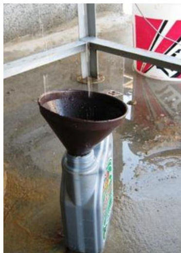
Figure (D.16): Measuring infiltrated water from pavement
