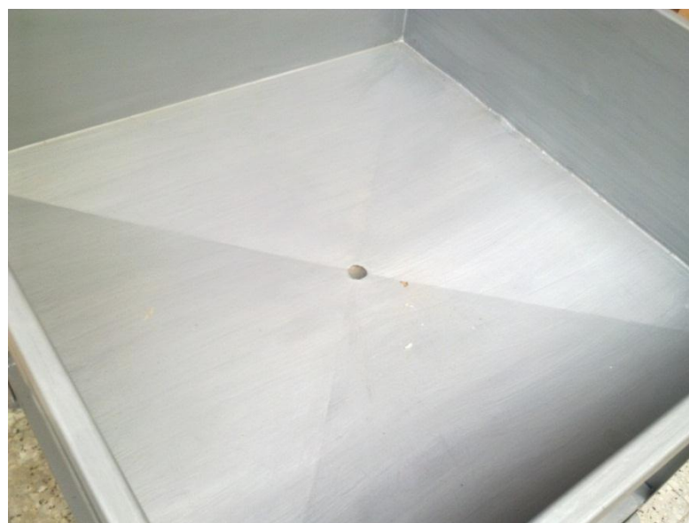
Figure (3.23): Infiltrated water collecting funnel
