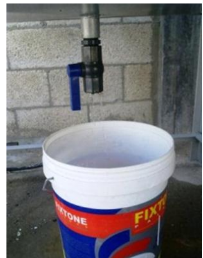
Figure (D.16): Measuring infiltrated water from pavement
