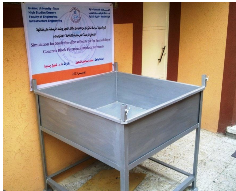
Figure (3.17): The experimental steel box of the permeable pavement
