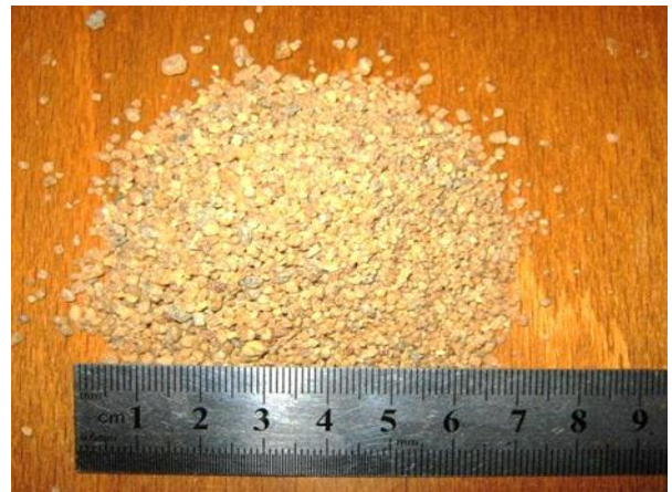
Figure (D.10): Filling material between joints
