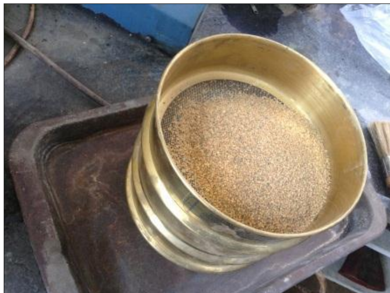
Figure (3.11): Sieve analysis for aggregate between joints (0/2.36)
