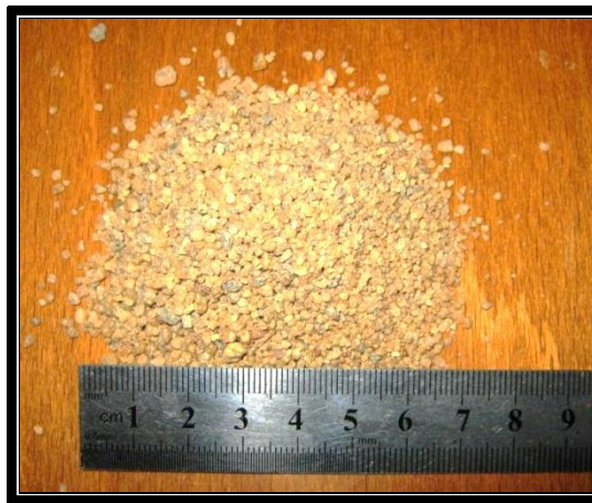
Figure (3.9): Filling material between joints
