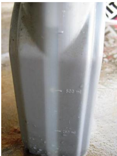
Figure (D.16): Measuring infiltrated water from pavement
