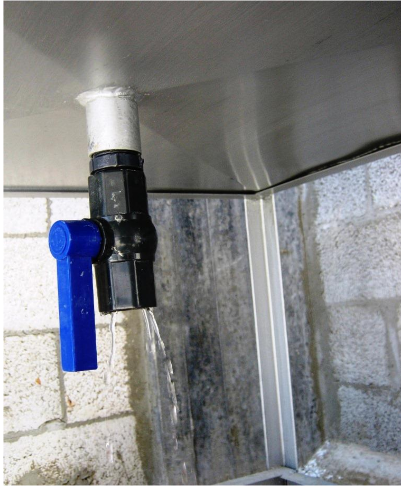
Figure (3.26): Infiltrated water out through permeable pavement
